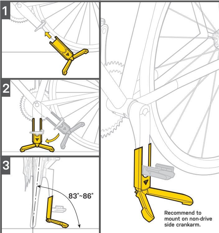
**Adjust FlashStand Slim X height to make sure your bike is within the recommended angle of 83°~86° (from horizontal plane) for stability of your bike.**
