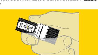
**IMPORTANT NOTE:** Hold the Torq Rocket at position shown when applying torque to achieve highest accuracy.
